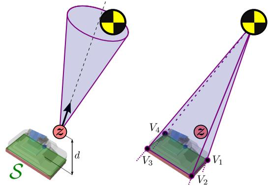
Fig. 1. The two necessary and sufficient conditions for contact stability of the Floating-base Inverted Pendulum. **Friction (left):** the COM belongs to the contact friction cone  $\mathcal{C}$  projected from the ZMP  $z$ . **Center of pressure (right):** the ZMP  $z$  belongs to the cone projected from the COM and containing the vertices of the contact surface  $\mathcal{S}$ .
