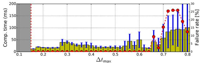
Fig. 2. Effect of  $\Delta t_{\max}$  on computation times (yellow) and failure rate (red) of the NLP solver, for a feasible step and  $N = 10$  collocation points. Each bar includes a standard deviation estimate (blue line) computed over 200 runs. Above a minimum value  $\Delta t_{\max}^{\text{lim}}$ , the problem becomes feasible and all runs should ideally converge to a solution. In practice, computations become unstable for large values of  $\Delta t_{\max}$ .
