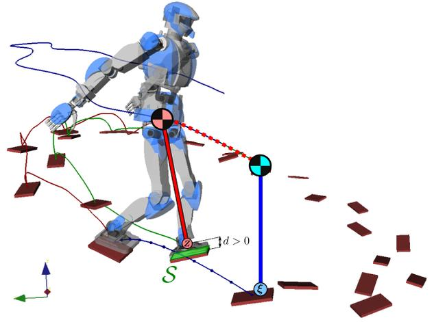
Fig. 3. **Walking pattern generation over an elliptic staircase with tilted steps.** At each control cycle, a new trajectory (dotted line) is computed via nonlinear optimization for the Floating-base Inverted Pendulum (red: current state, blue: desired state at the end of the receding horizon). In this model, the ZMP  $Z$  can leave the surface patch  $S$  and the COM can move freely in 3D while keeping linear equations of motion.
